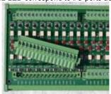
Easy exchange by interchangeable screw-terminals
